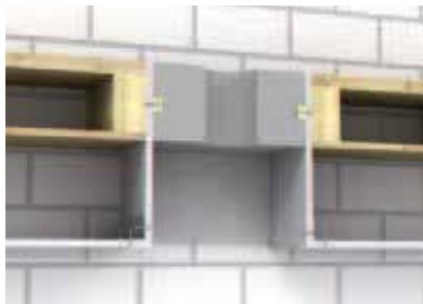
Wooden beam ceiling with classified ceiling substructure
